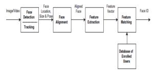
Figure 1: Face Recognition processing flow
