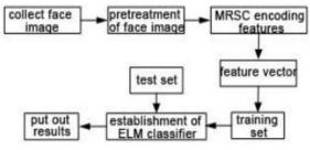
Figur3.Workflow of Face Recognition Method
